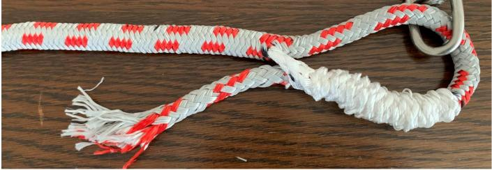
Hold the crossover firmly and milk the core until cover disappears.
