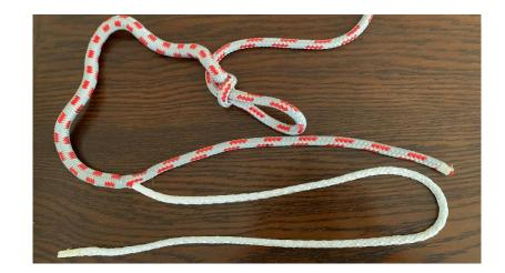
Milk cover to knot & back twice. Mark the core where it leaves the cover.
