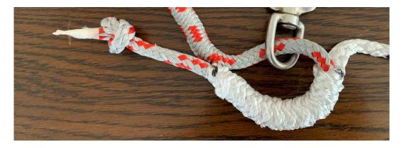
At the first mark push **smaller** fid into cover past join at the short fid mark and out through cover. Insert core into fid and push through.
