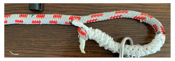
Undo the cover knot, fan and taper the end of the cover.
