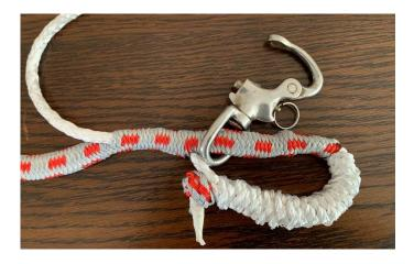
Mark the core where it leaves the cover. Pull out the core, cut at the mark, taper the end.
