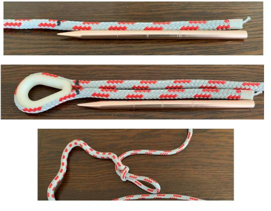
At the second mark use a spike to carefully open the cover & remove core, tape the end.
