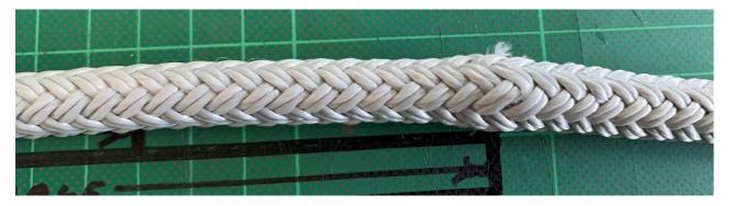
Stitch and whip the joint on the side of the core and continue the stitching through the cover end.
