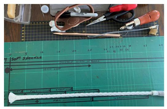
Cut the core and milk the cover back and feel for the end of the core.
