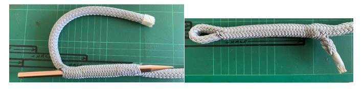
Remove the tape and milk the cover until the end meets the end of the core
