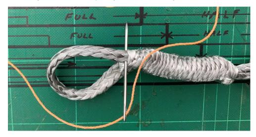
Milk the cover back and tie the ends of the light line into a loop.
