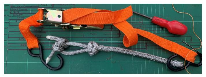
To make the shackle easier to reuse a light line may be added as a quick release. Milk the cover back and pass a light line through the core. You may recognise this as crabbing line!
