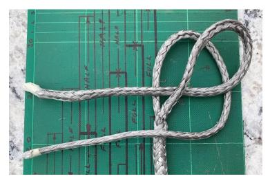
Continue over the standing part, under the free end, over the loop, under itself and over the loop. This forms the carrick bend.
