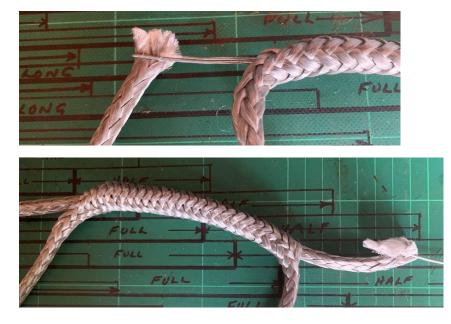
Put a fid or spacer in the loop to prevent it closing and pull it tight.
