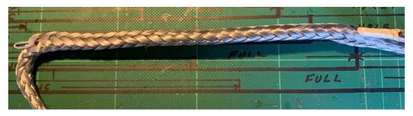
Put the long end into the wire loop and start to pull it through.
