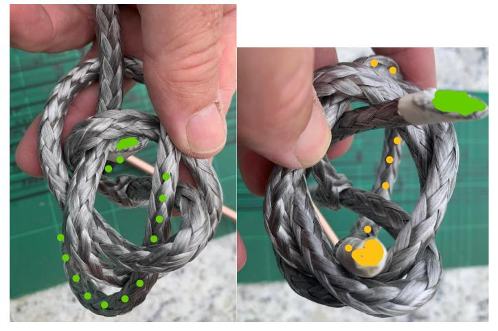
Dress the knot close to the splice and tighten as much as possible. Spike, pliers, ratchet strap or winch may be used.
