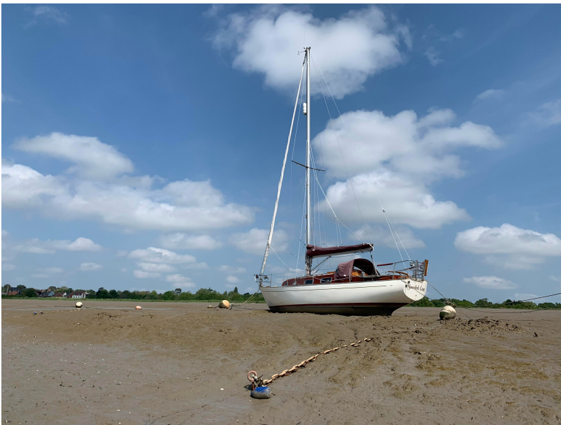
Completed ground chains (1m of tide)
