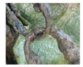
A timely reminder of how the creek mud is an excellent grinding paste. This chain was removed from a mooring in September.
