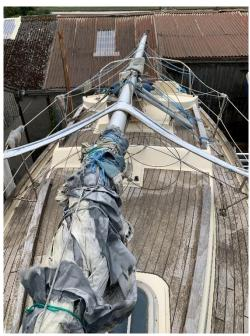
The decking is laid on West system resin rather than screwed. The foredeck has fairleads on the rail and a samson post. She has an anchor well with chain, fisherman and a plough type anchor.
