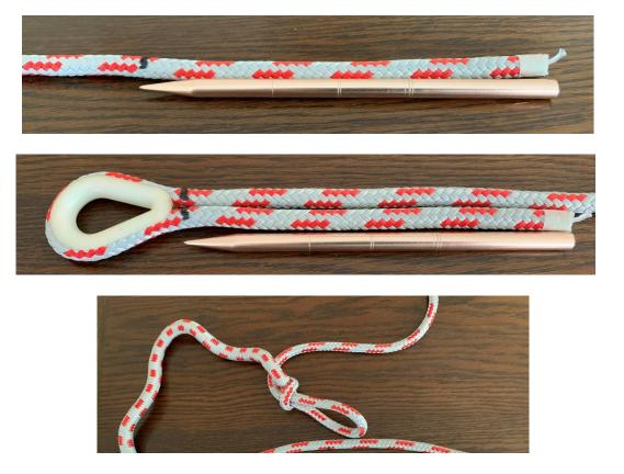
At the second mark use a spike to carefully open the cover & remove core, tape the end.
