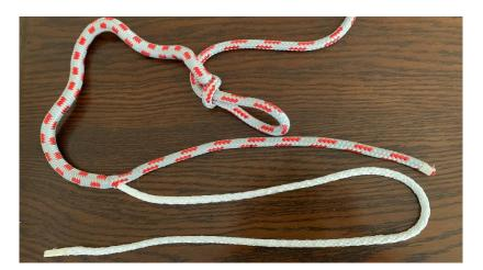
Milk back to expose more core in order to mark a short fid length & a further 1.5 fid lengths.
