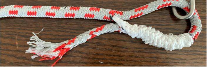
Hold the crossover firmly and milk the core until cover disappears.
