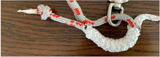
At the first mark push **<u>smaller</u>** fid into cover past join at the short fid mark and out through cover. Insert core into fid and push through.
